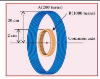
Solution:  $N_A = 200$ ;  $N_B = 1000$ ;  $r_A = 20cm = 20 \times 10^{-2} m$ ;  $r_B = 2 cm = 2 \times 10^{-2} m$  $di_A = 6 - 2 = 4 A$ ; dt = 0.04 s;  $M_{BA} = ?$ ;  $\epsilon_B = ?$
